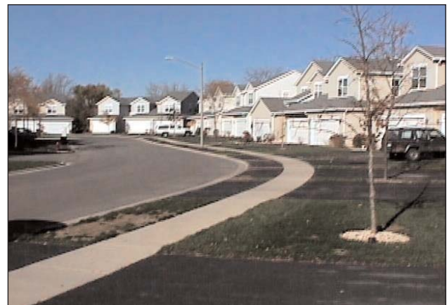
Wide roads in conventional residential development developments increase runoff and air temperature and encourage higher speed traffic.
