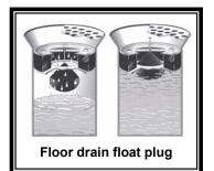
One variation is a plug with a float. It allows water to drain out of the basement (see illustration, left side). When the sewer backs up, the float rises and plugs the drain (see illustration, right side). A
