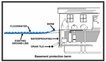
basement walls and the surrounding soil. This will greatly increase the amount of water pressure against the basement walls.
